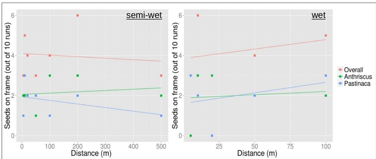
**Figure 3.4.** Seed attachment on the bike frame including regression lines. The x-axis shows attached seeds out of the ten runs for the particular distance. The y-axis represents the distance in which the numbers were recorded. Red: Overall seeds, green: *Anthriscus*, blue: *Pastinaca*.
