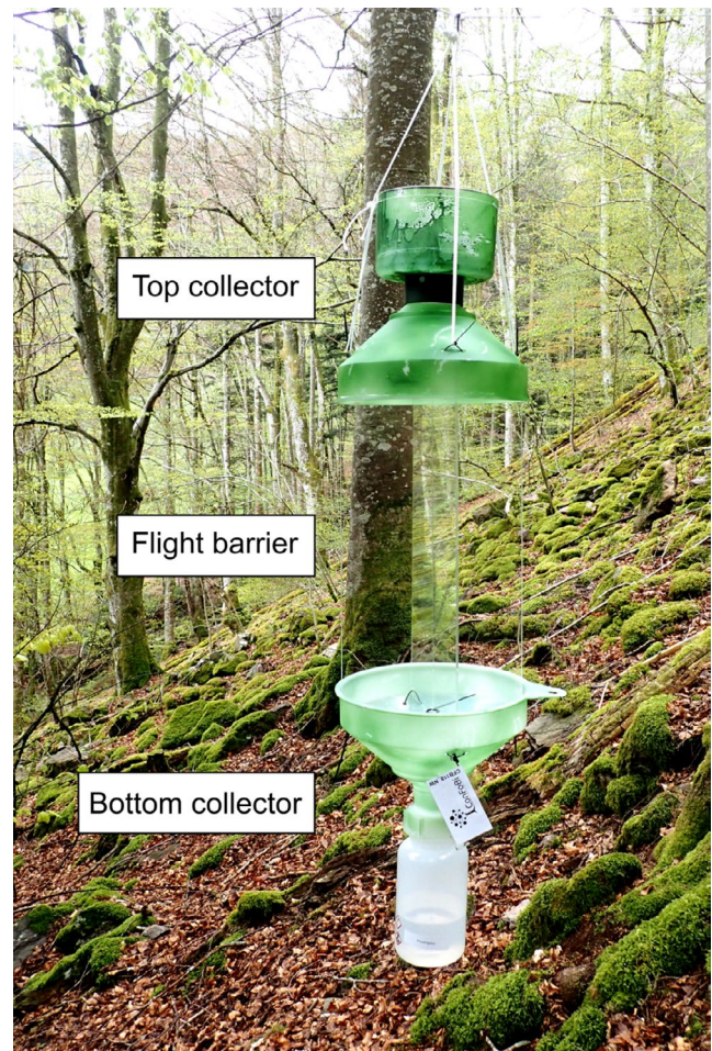
FIGURE 1 Modified window trap supplemented with top collection unit. Two transparent crossed windows serve as flight barrier. Funnels beneath and on top of the windows serve as sturdy attachments between windows and collectors and direct arthropods into the collectors. For details see Supporting Information S1
